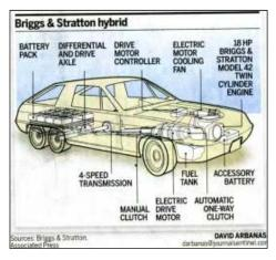
If you think the gasolineelectric hybrid automobile is a recent invention, think again. In 1979 the Briggs and Stratton Co. developed a hybrid, not to sell, but to demonstrate that the technology, even then, was capable of the task. The car could go up to 70 mph, had a fiberglass body, a third set of wheels to support the battery
